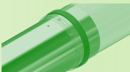
2) ACCOSTARE I DUE TUBI INNESTANDO LA BULINATURA DI BLOCCAGGIO (A) DEL TUBO MASCHIO, NEI CANALI DI GUIDA (B) DEL LATO FEMMINA.
